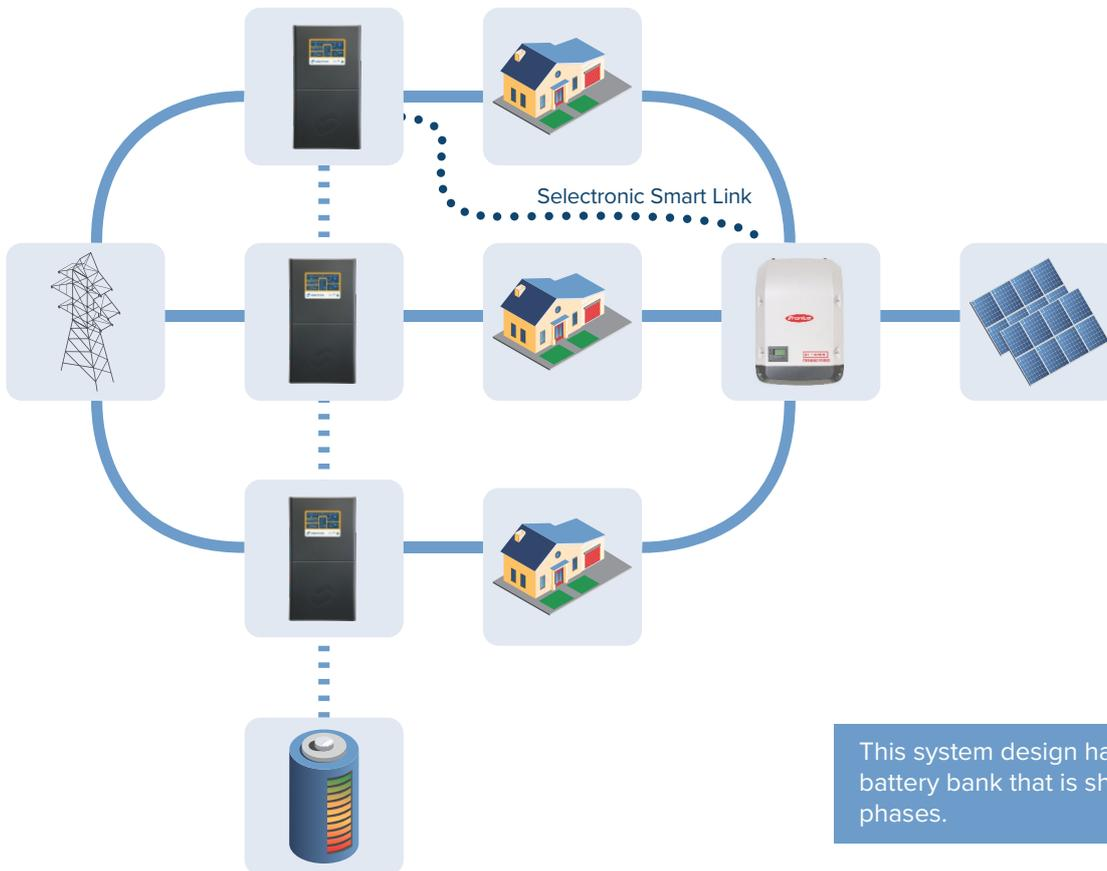
This system design has one common battery bank that is shared between phases.
