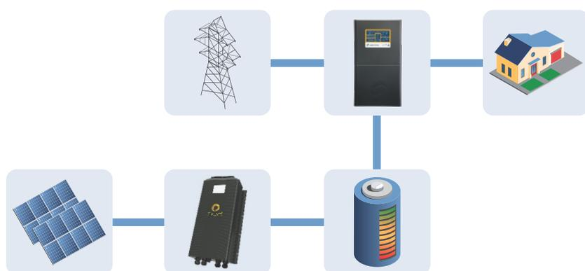
This system design uses an MPPT (Maximum Power Point Tracker) solar controller in place of a solar inverter.
